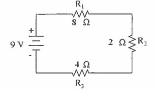
b. What is the total equivalent resistance of the circuit?
